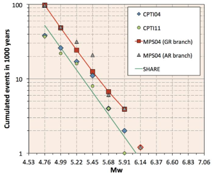
**Figure 3.** Comparison between the cumulative number of earthquakes in the CPTI04 and CPTI11 catalogs and the seismicity rates for the GR and AR branches of MPS04 and for the SHARE project (as available on July 2012) for seismic source zone 912. All rates are normalized to 1000 years.
